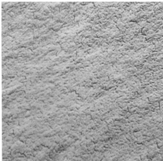
Figure 1 The surface of uncrosslinked PE (Magnification x6000)
