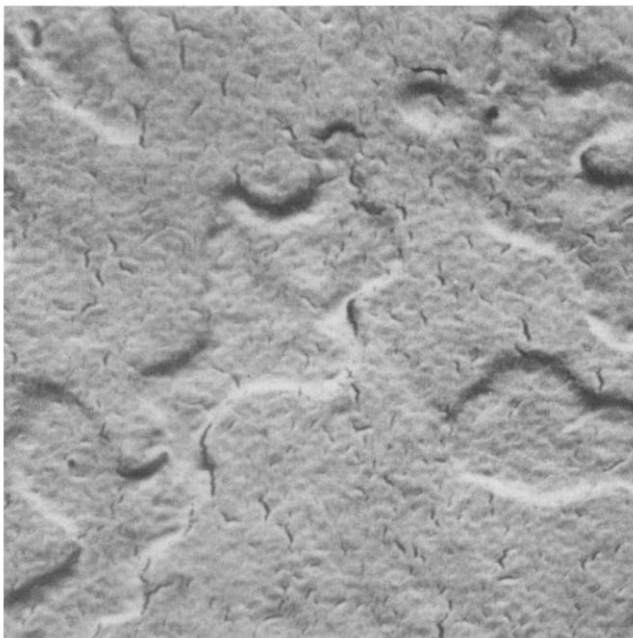
Figure 2 The surface of crosslinked PE with 61% of gel fraction (magnification x6000)
